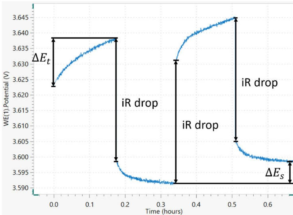
**Figure 3.** First two charge steps, each composed by 10 minutes of C/10 galvanostatic charge, followed by 10 minutes of relaxation time. The iR drop is shown, together with the  $\Delta E_t$  and  $\Delta E_s$ .
