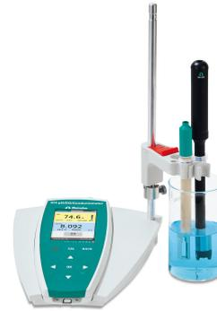
Figure 1. 914 pH/DO/Conductometer O<sub>2</sub>-Lumitrode
