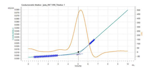
Figure 2. Example titration curve to determine the total base number in motor oil according to IP test method 400.
