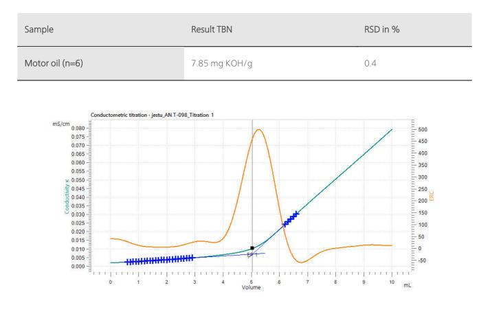
Figure 2. Example titration curve to determine the total base number in motor oil according to IP test method 400.
