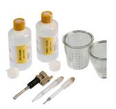
Complete electrode set for the determination of organic additives in electroplating baths with CVS (Cyclic Voltammetric Stripping). Contains rotating platinum working electrode (electrode diameter: 2 mm), reference electrode, platinum auxiliary electrode, measuring vessels and electrolyte solutions.
