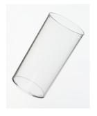
Reaction vessel for stability measurements with Rancimat and PVC Thermomat. Set of 117 pieces.
