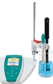
**Figure 1.** 914 pH/DO/Conductometer equipped with an O<sub>2</sub>-Lumitrode and conductivity sensor for the determination of dissolved oxygen in wine samples.
