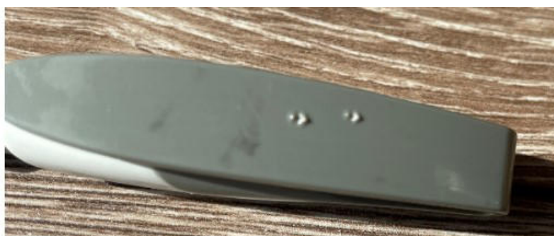
Figure 3. Grey plastic pen, burned with a 1064 nm system and identified as polystyrene with MIRA XTR DS.
