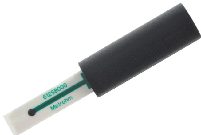
The scTRACE Gold sensor holds all three electrodes required for a voltammetric determination. Together with the electrode shaft it makes a complete electrode system which can be used in any Metrohm voltammetric measuring stand. No further electrodes are required. The working electrode is a gold microwire. Reference and auxiliary electrode are screen-printed electrodes.
