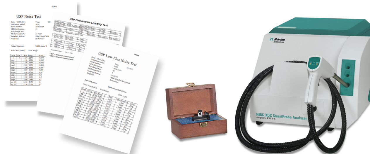
Figure 2. Report of the USP Wavelength Accuracy Test from Vision software (left) and used Metrohm NIRS XDS SmartProbe Analyzer with standard (right).
