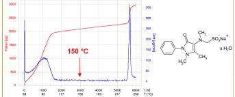
The water release curve was recorded using a heating rate of 2 °C/min.
