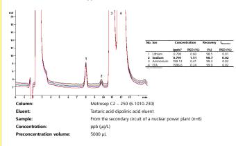
The recovery rate of the investigated cations ranged from 98.5 to 99.9%. Interfering adsorption and contamination processes related to the vessel walls are minimized by using very large sample vessels (up to 500 mL). Additionally, timeconsuming and error-prone decanting procedures are avoided.
