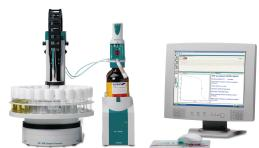
The preliminary titrations showed markedly delayed endpoint detection. After titration of the released moisture, reagent consumption continued, indicating a retarded water release from the sparingly soluble cellular cocoa matrix or iodine-consuming side reactions. Since the removal of the cellular matrix had no effect on the titrant consumption, the first
