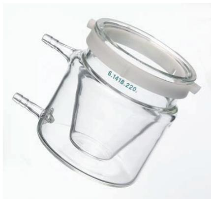
Heatable cell for titrations at elevated temperatures
