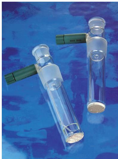
Generator cells for Metrohm KF Coulometers:
