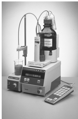
Microprocessor-controlled piston buret Used for automatic titrators and as buret with multiple dosing programs.
