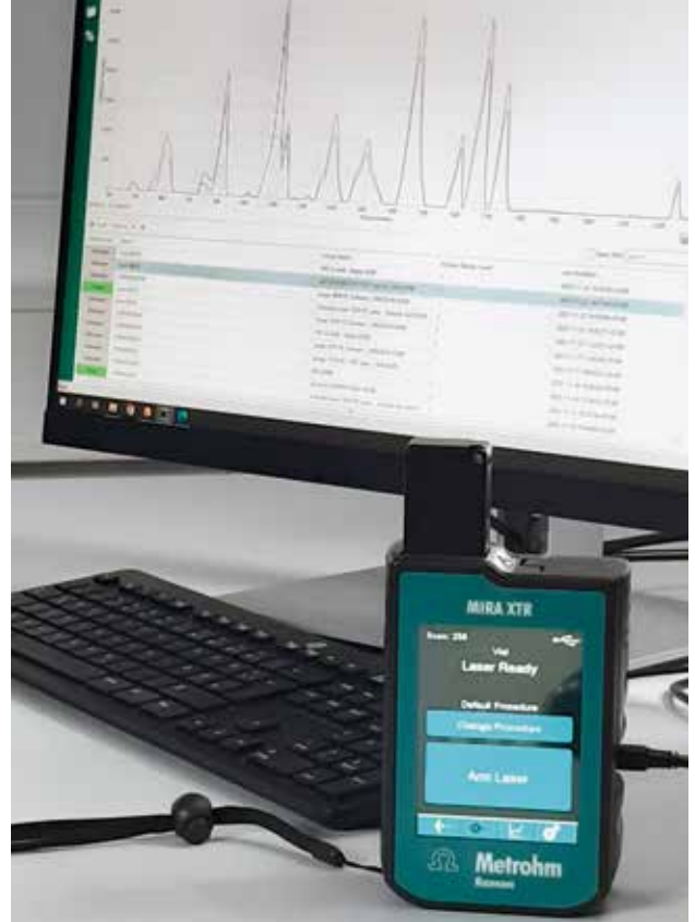
Thanks to the XTR algorithm, MIRA Cal Software can extract a clear Raman signal even from colored and black polymers.
