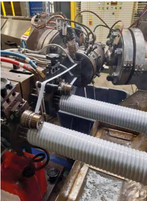
Production of polymer pipes by extrusion at Hauff-Technik in Hermaringen.
