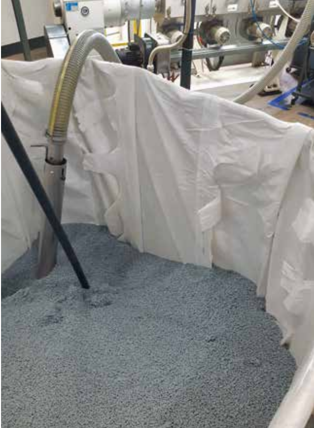
Polymer pellets are fed to one of Hauff-Technik's extruders in Hermaringen.
