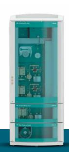
940 Professional IC Vario with conductivity and amperometric detection. The high-pressure gradient system is extendable with the 942 Extension Modules to up to a quaternary high-pressure gradient system or the 941 Eluent Production Module.
