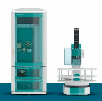
940 Professional IC Vario with the 947 Professional UV/VIS Detector Vario SW, a 943 Professional Reactor Vario, and a 858 Professional Sample Processor for automated sample handling.
