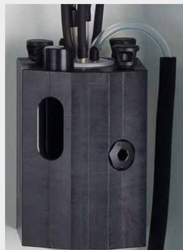
(L) Thermostated cuvette module at the heart of the 2029 Process Photometer. (R) Drift-controlled measured value acceptance.
