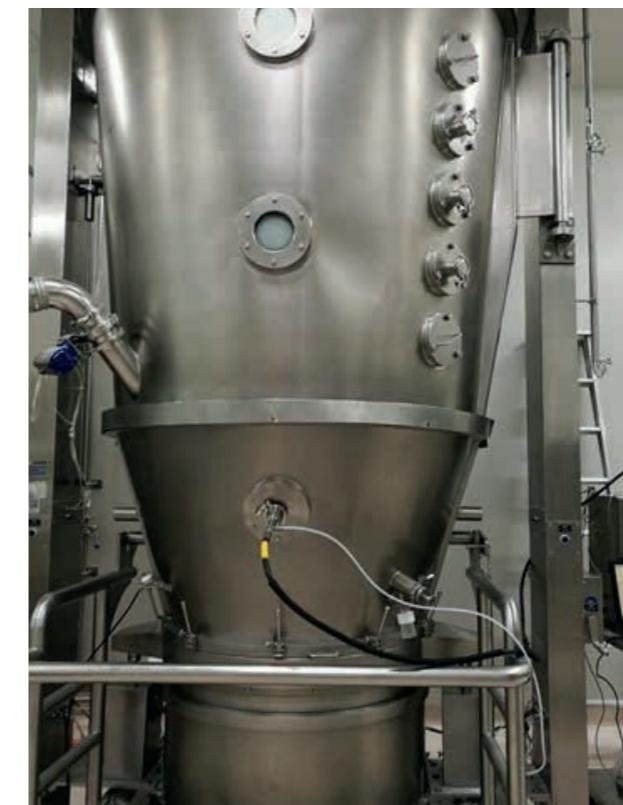
Spoon probe implemented in a dryer
