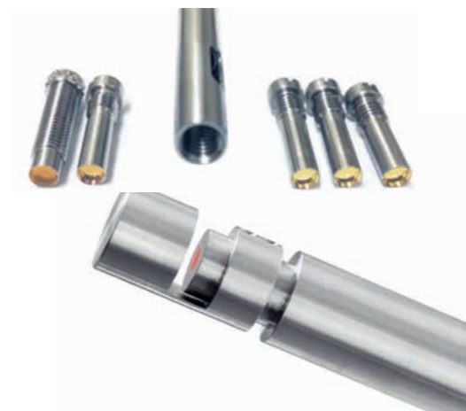
Top: Single fiber transfection probe with a set of mirrors for defined OPL (left to right): 0.5 mm, 1 mm, 2 mm, 5 mm, 10mm. Bottom: Microbundle fiber transfection probe with adjustable mirror
