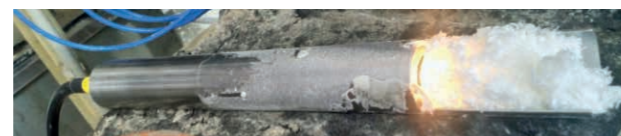
Example of non-contact probe inserted in an outer sleeve for fluffy samples
