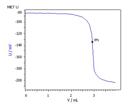
Cobalt can be analyzed using the Cu ISE. A small amount of Cu-EDTA complex thereby acts as indicator as the Cu ISE itself is not sensitive for cobalt.
