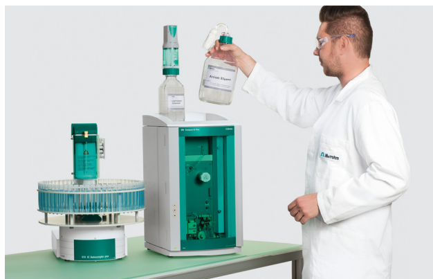
Figure 1. Instrumental setup including a 930 Compact IC Flex, 919 IC Autosampler plus, and an 800 Dosino for automatic regeneration of the Metrohm Suppressor Module (MSM).
