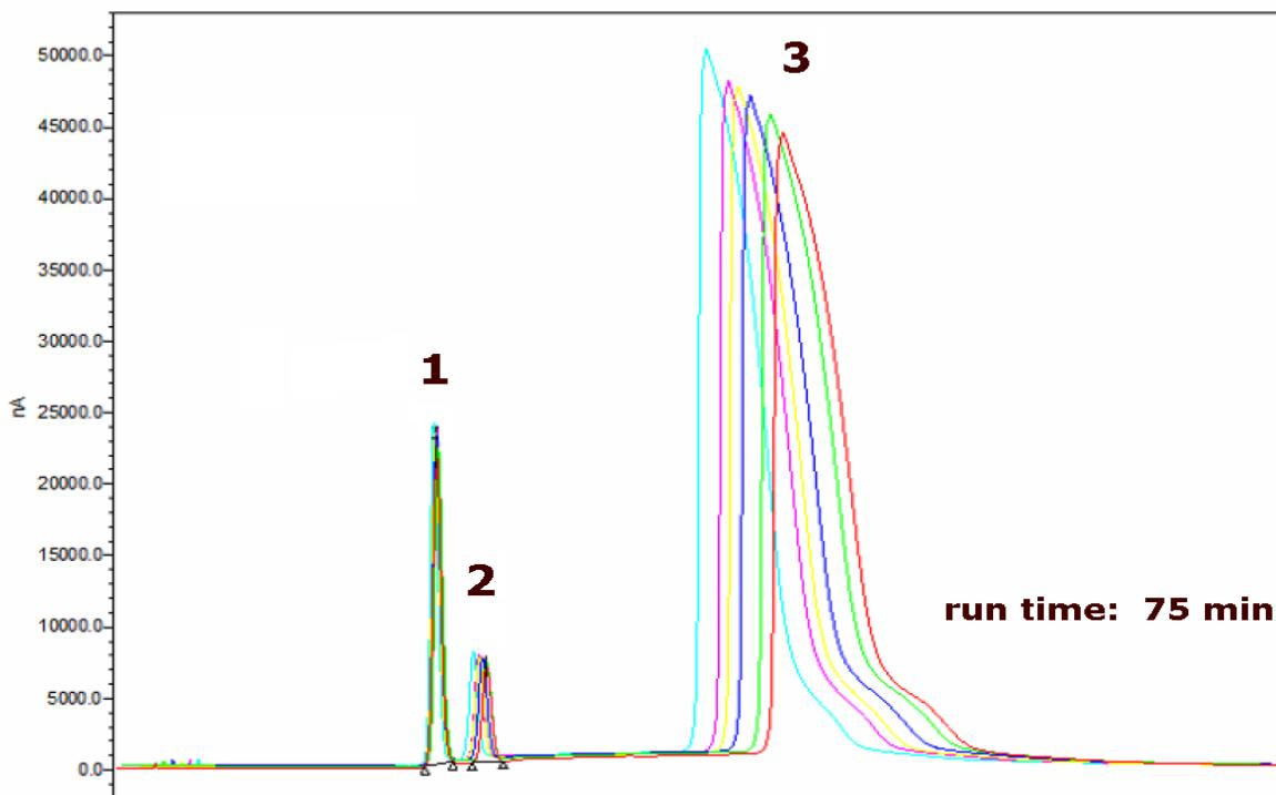
This Application Note shows the determination of glucose and galactose in a 2% solution of lactose. The separation is achieved on a Hamilton RCX-30 - 250/4.6 applying pulsed amperometric detection (PAD) at a gold electrode. Instrument control, data acquisition, and data handling is done by Empower 3.0 using the Metrohm IC Driver 2.0 for Empower.
