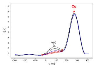
The example shows the determination of 10.8  $\mu$ g/L As(V) besides approx. 50  $\mu$ g/L Cu in a ground water sample. An excess of Cu can cause false low readings for arsenic (in the above example the recovery was only about 70%) or can even completely hide the As peak.
