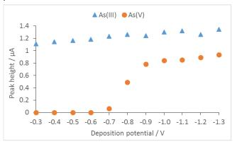
For the determination of As(III) the deposition potential should not be more negative than -0.6 V otherwise also As(V) is partly reduced and deposited.
