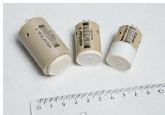
All three suppressor rotors – MSM-HC, MSM, and MSM-LC – have the same design and vary solely in terms of their capacity.
