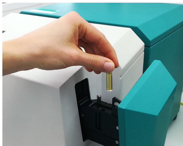
Figure 1. XDS RapidLiquid Analyzer with 8 mm disposable vial filled with a diesel sample.
