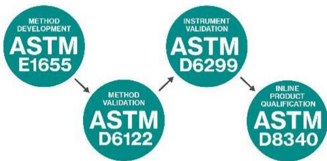
Figure 2. Different steps for the successful development of quantitative methods according to international standards.
