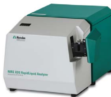
Figure 1: The NIRS XDS RapidLiquid Analyzer was used for spectral data acquisition over the wavelength range from 400 nm to 2500 nm.
