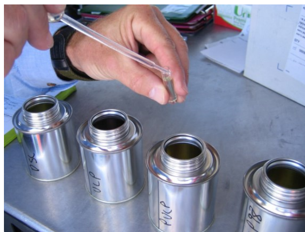
Figure 1. Samples filled in disposable vials with 8 mm path length.
